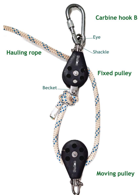
Figure 2 The hauling system set up.
