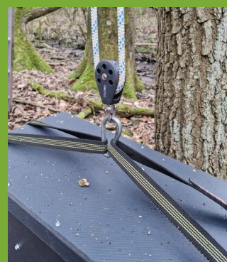
Figure 19 Moving pulley clipped into hauling sling.
